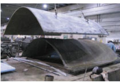
Fig. 17. Step 4 – Thin-shell funicular GFRP vault produced from mold (C.A.S.T. photo)
