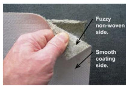
Fig. 18. Fabric for forming rigid molds (C.A.S.T. photo)
