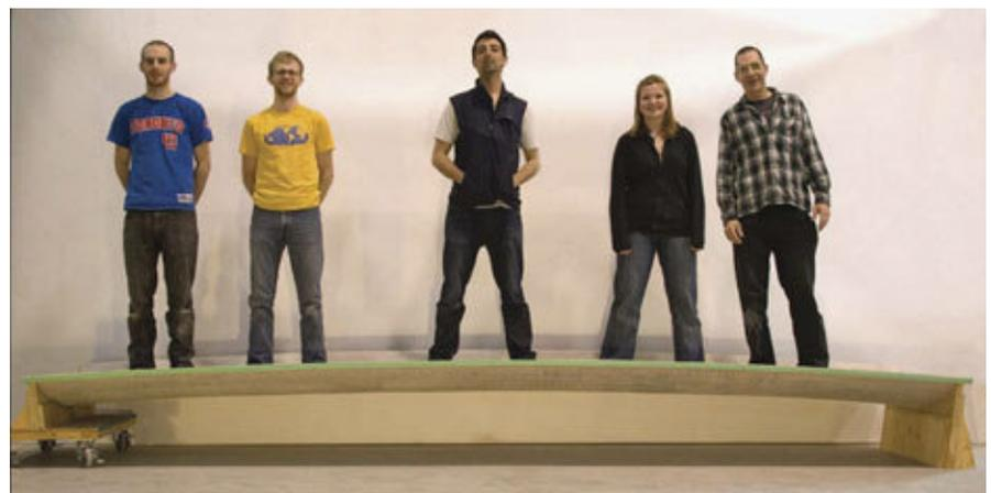
Fig. 21. Completed double curvature funicular thin shell vault (C.A.S.T. photo)
