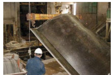
Fig. 16. Step 3 – Resulting funicular shell is inverted to form mold (C.A.S.T. photo)
