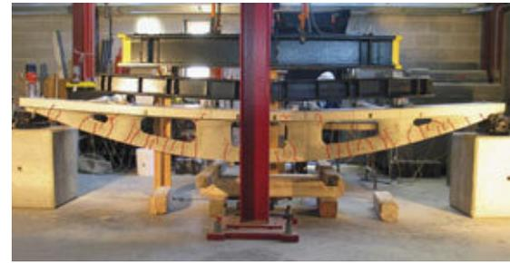
Fig. 13. Testing of variable section concrete truss (C.A.S.T. photo)
