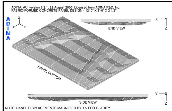
Fig. A2. Final concrete panel shape using FEA.
