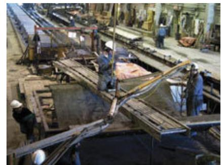
Fig. 15. Step 2- Uniform layer of GFRC is applied (C.A.S.T. photo)
