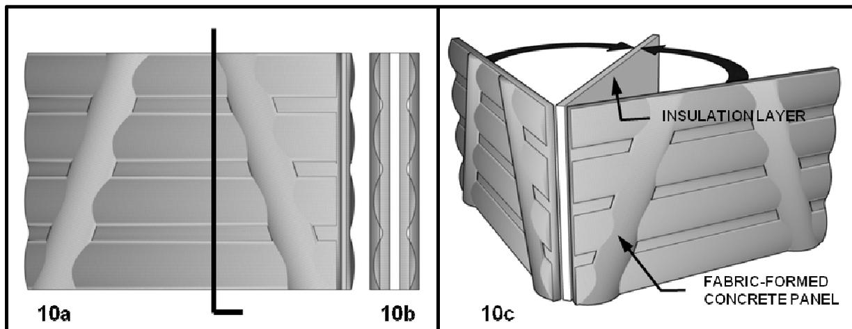
**Figure 10. Computer aided design drawing of a fabric-cast wall panel system (Figures by RPS).**
