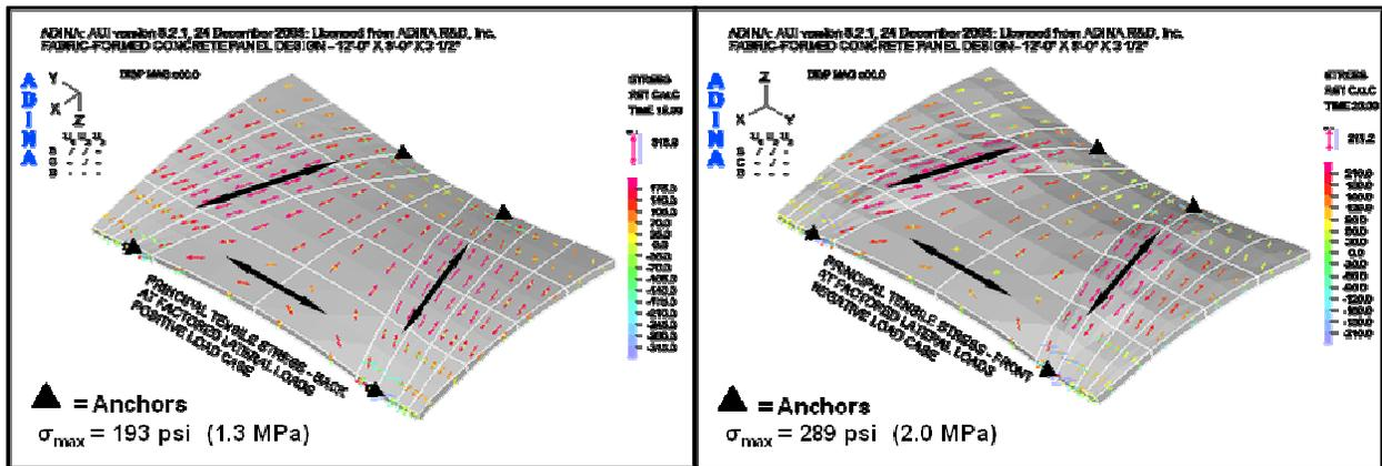
Figure 6. Panel principal stresses, back (left) and front (right) (Figures by RPS).
