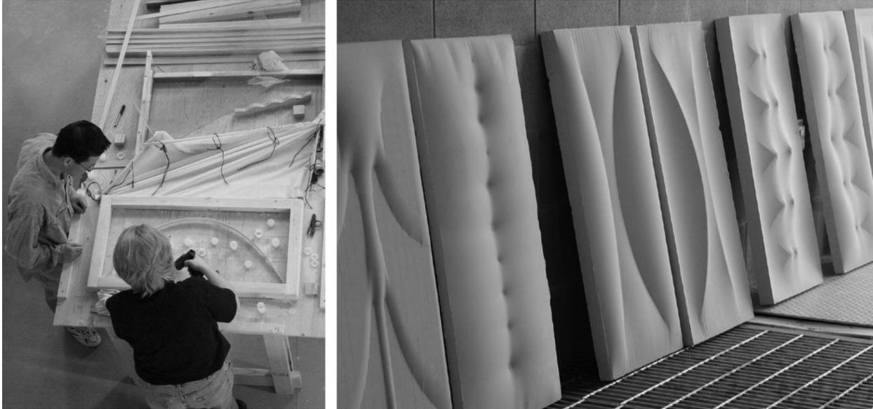
**Figure 3. Model formwork and completed plaster cast (C.A.S.T. photos).**
