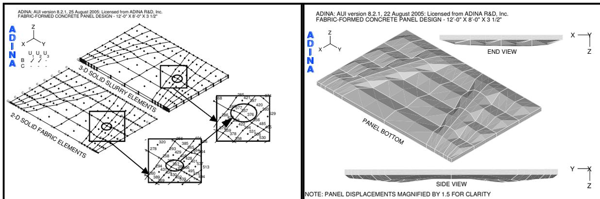
**Figure 5. "Form-finding" combined fabric and slurry model (left), resultant panel shape (right) (Figures by RPS).**
