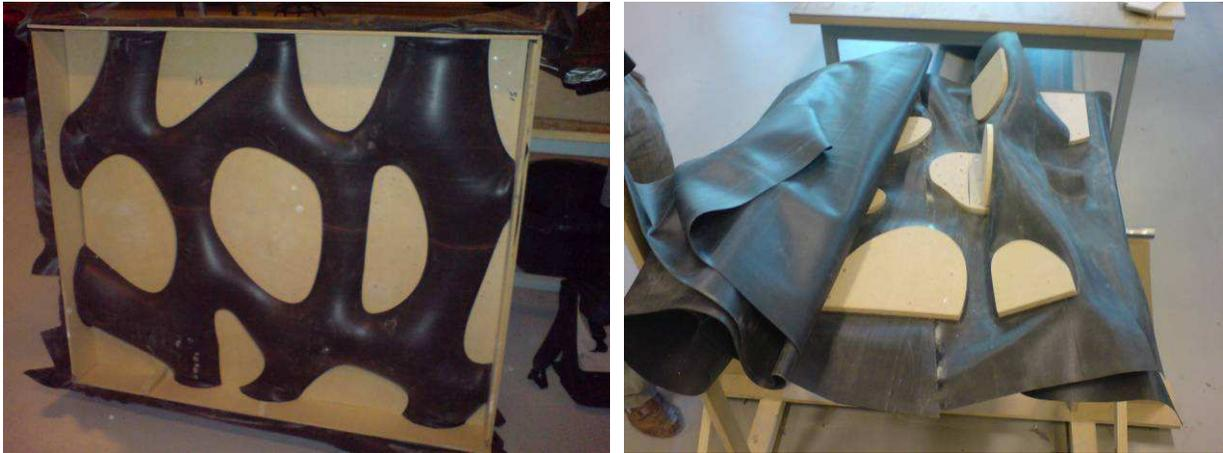
**Figure 16:** *Mould of façade element*
