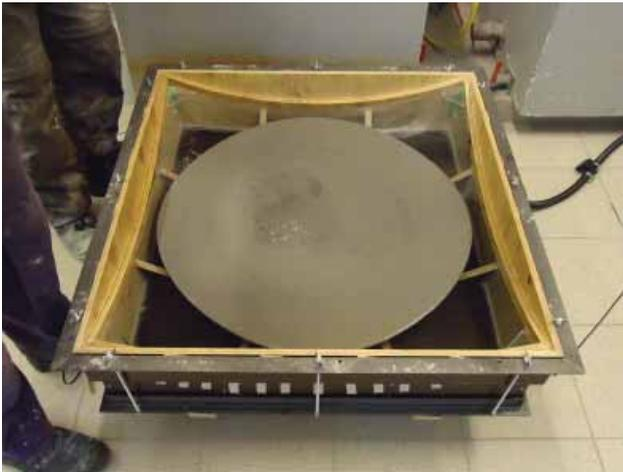
4-27: Wet concrete poured on bottom foil
