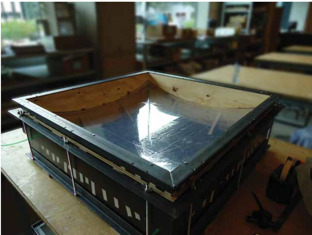
4-17: Assembled mould
