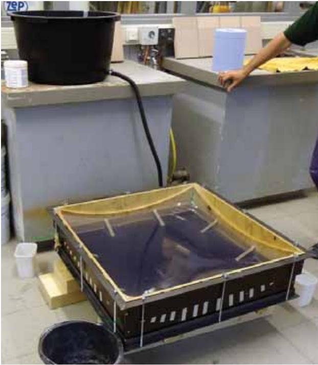
4-19: Filling the bottom mould with water
