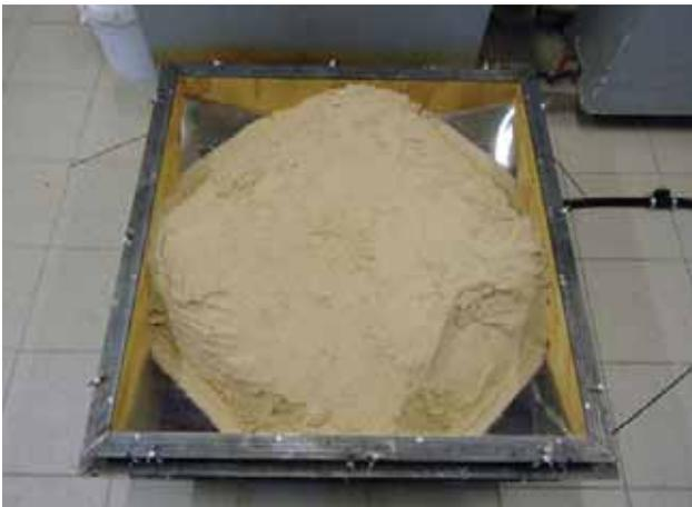
4-22: Top mould is loaded with sand
