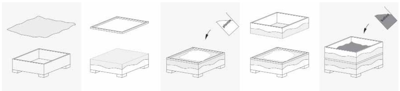
4-4: Process of casting plaster samples
