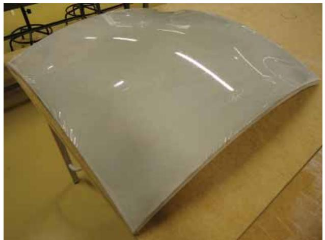
4-39: Underside of the grey segment with 'dents' in the corners
