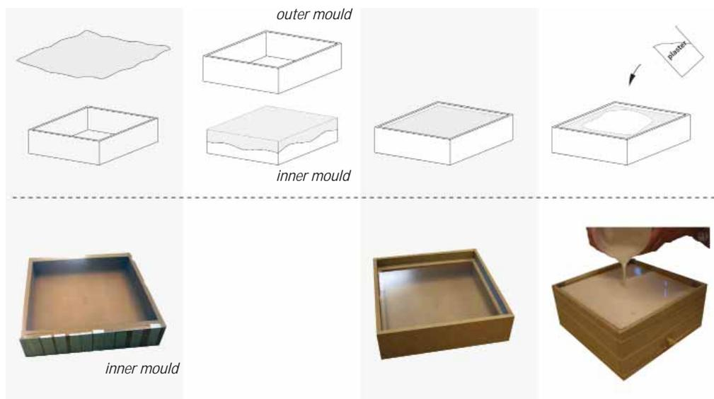
3-6: Process of casting plaster sample
