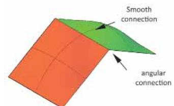
3-23: Connection between flat mould-segments
