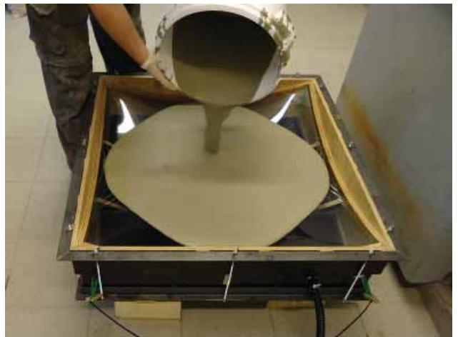
4-36: Grey concrete poured into the mould
