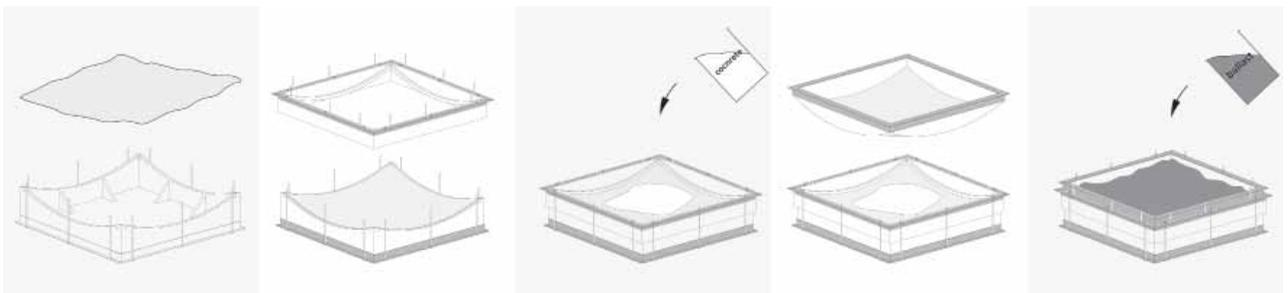
4-14: Process of casting concrete segments
