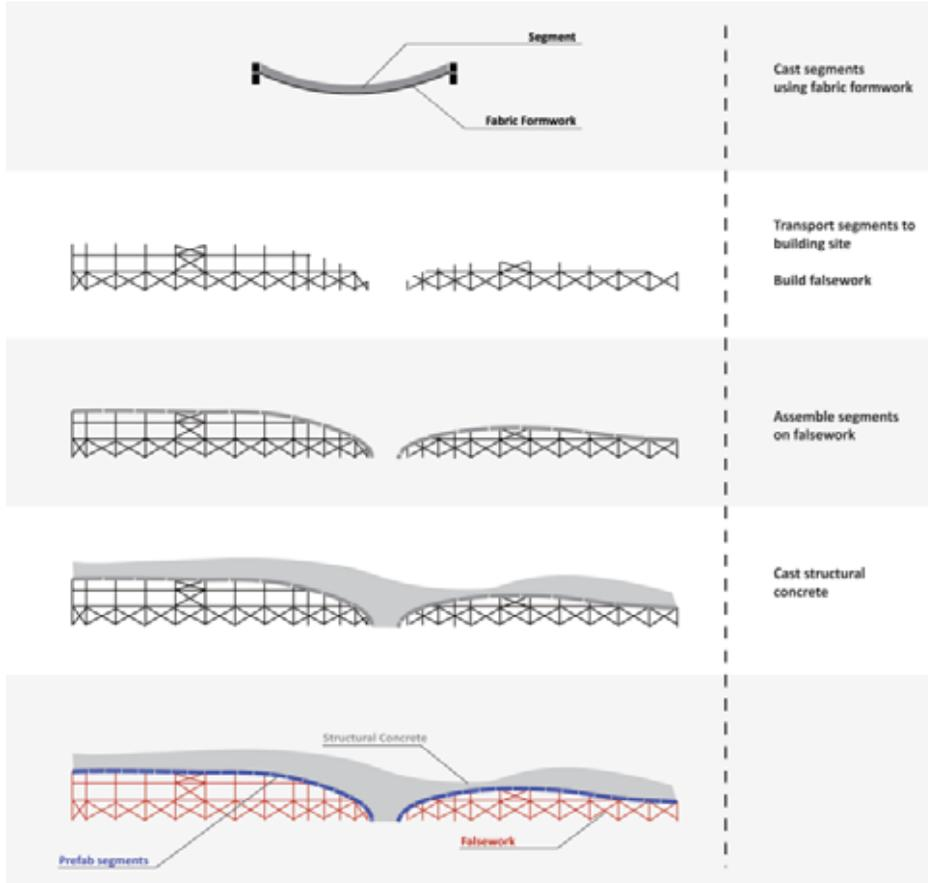
2-18: Building process with prefabricated fabric formwork
