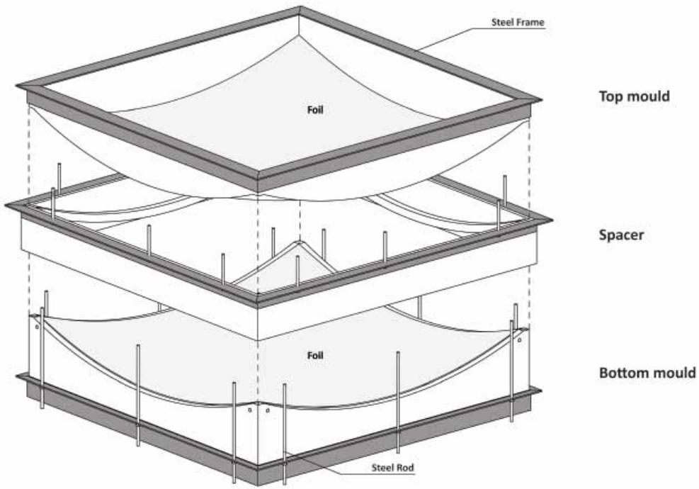
4-11: Exploded view of the mould
