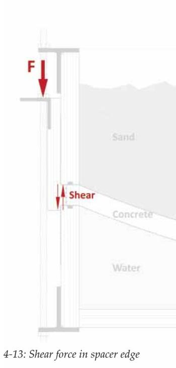
4-13: Shear force in spacer edge
