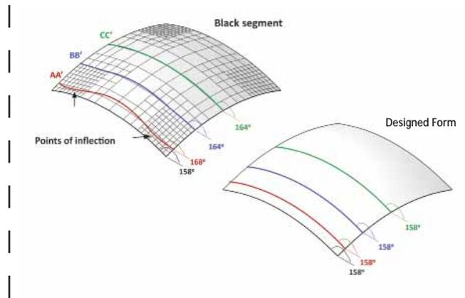
4-43: 3D-model of concrete segment (left) and designed form (right)
