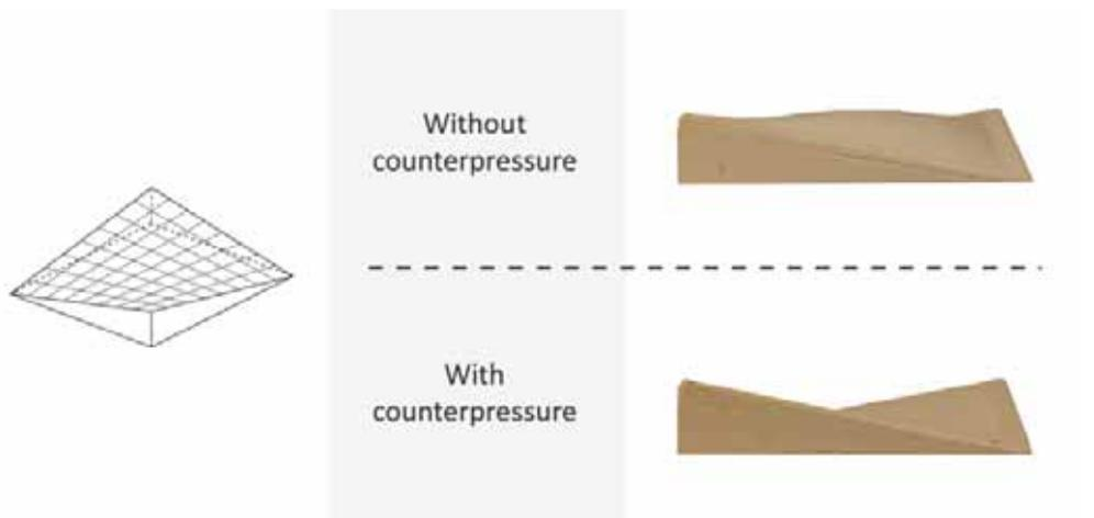
The form that was cast with counterpressure resembles the initial form of the (unloaded) foil. If this is actually the result of the counterpressure of the water, this is an important discovery. It would mean that it is possible to predict the forms that are cast in ‘curved moulds’: the forms are equal to the initial form of the foil. There are several pieces of software that can be used to calculate the form of loaded membranes.
