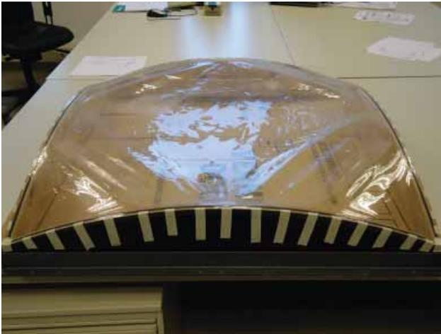
4-34: Plastic deformations in foil (before restretching)
