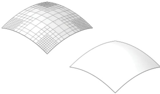
4-42: 3D-model of concrete segment (left) and designed form (right)
