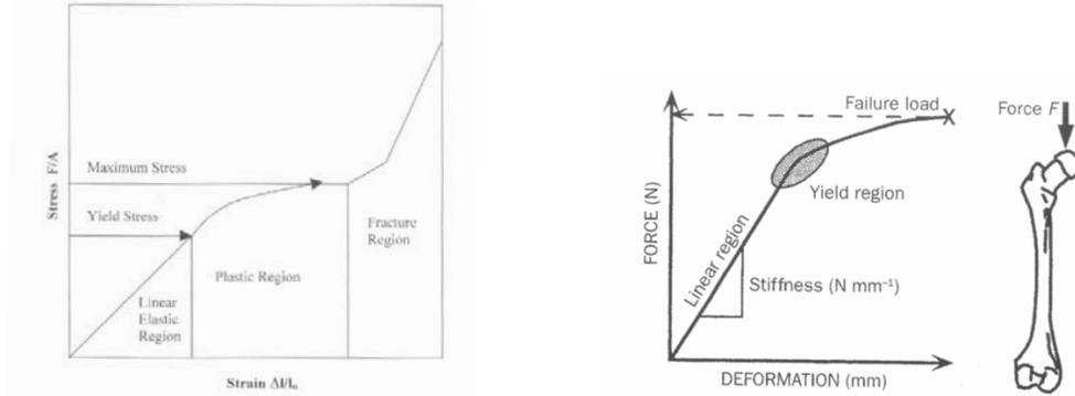
Figure 12: phases of mechanical properties
