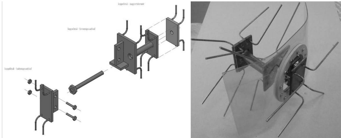
Figure 18: Anchoring the different sections
