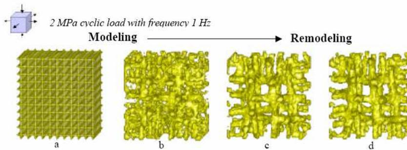
Figure 8: Process of forming the structure due to deformations
