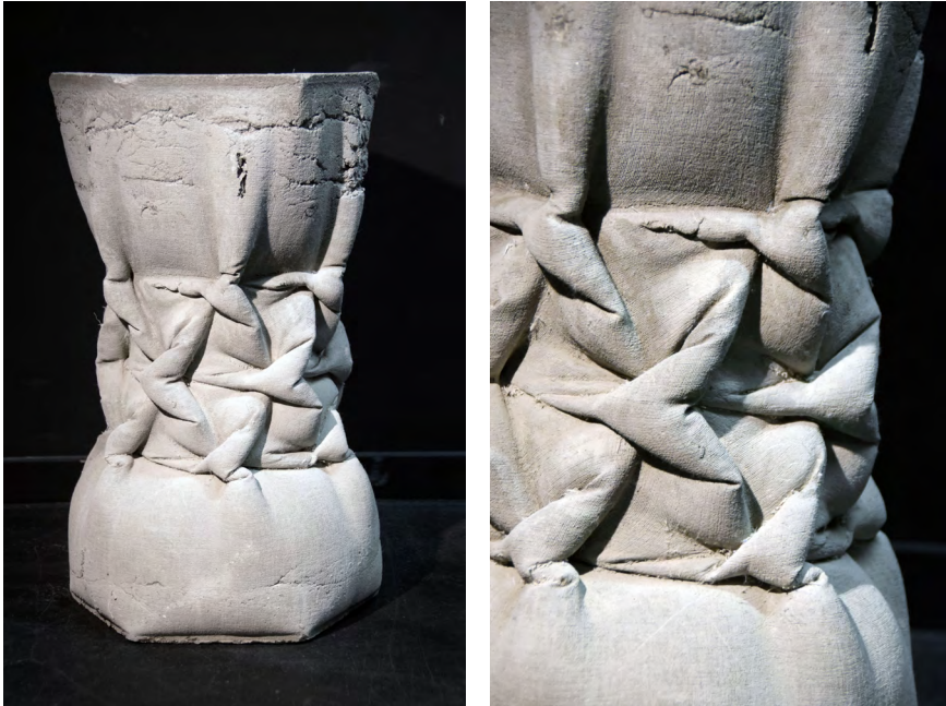
FIGURE 5.38: Column 3.2 cast prototype (Source: author).
