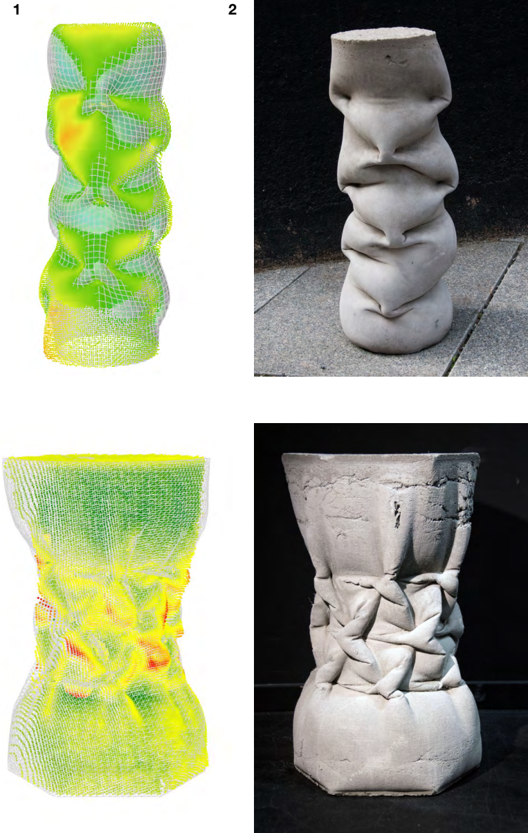
FIGURE 5.73: Column 02 and Column 3.2 : (1) simulation overlay with point cloud scan, colored for deviation and (2) cast prototype (Source: author).
