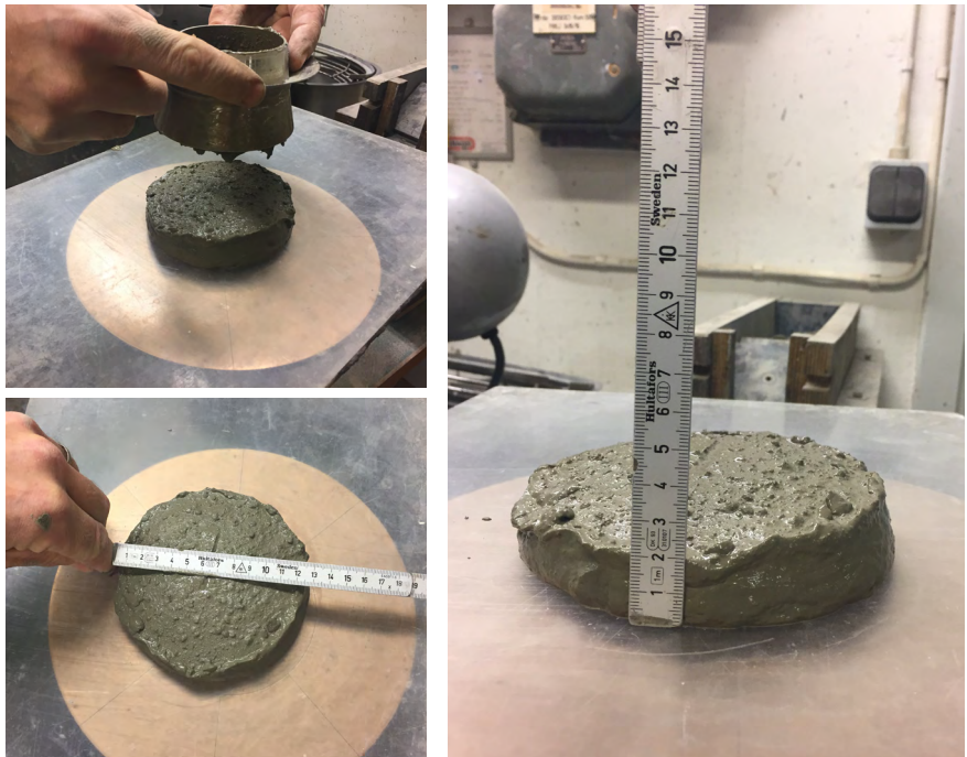
FIGURE 5.7: Concrete mixture ratio and slump tests (Source: author).
