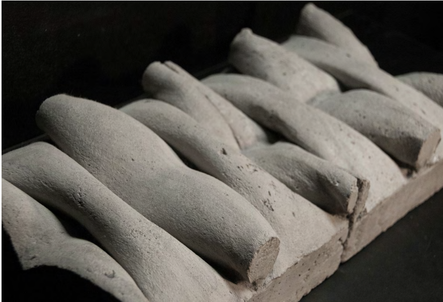
FIGURE 5.16: Cast Lozenge Panels . Left and right are felt and tarpaulin, respectively (Source: author).
