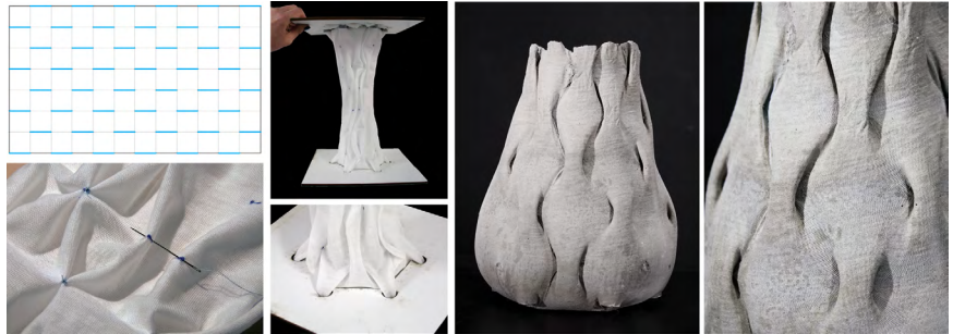
Figure 3 Column 1 lozenge smocking pattern, fabric formwork, and cast probe
