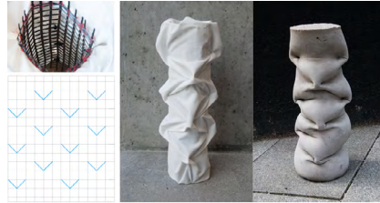
Figure 4 Column 02 basic arrow smocking pattern, formwork, carbon fiber reinforcement grid and cast probe
