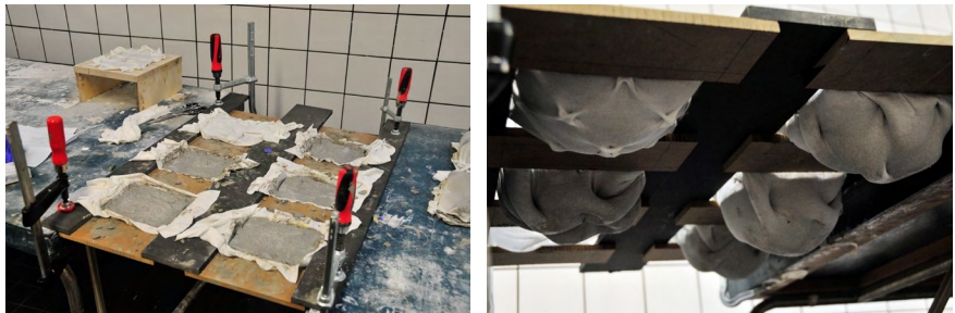
FIGURE 5.1: First Fifteen Hand-Smocked Probes casting setup (Source: author).
