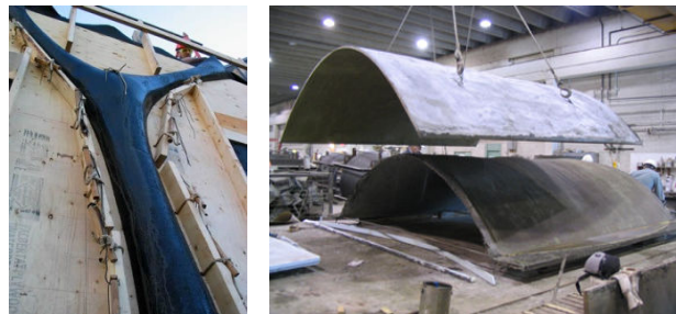
Figure 2: (left) Fabric formwork for a beam with expressive, natural curvature [4]. (right) Simple vault cast on fabric formwork [4].
