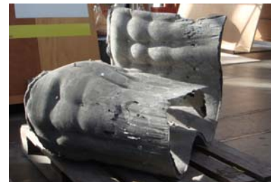
Figure 6: Chair cast in fabric formed concrete. The formwork blew while casting.
