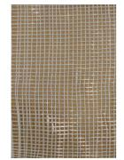
Fig. 1a 2D glass fibre textile
