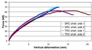
Fig. 5 Vertical deformation at shell centre in function of total applied load
