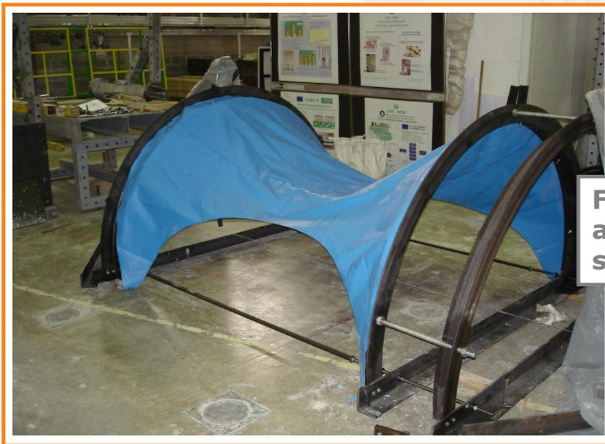
**Fabric formwork allows for a great shape flexibility**
