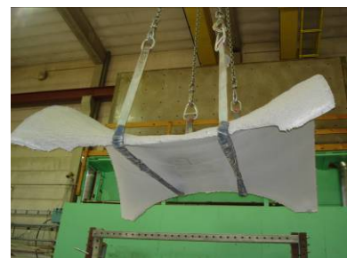
Fig. 10: Shell after demoulding.
