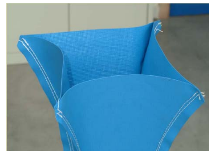
Fig. 4: Stitched column head
