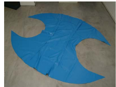
Fig. 7: Fabric formwork for the double-curved shell.
