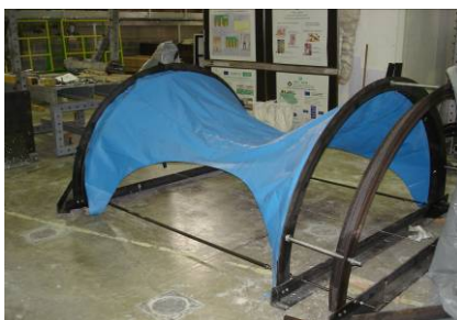
Fig. 8: Pretensioning the fabric with a secondary structure.
