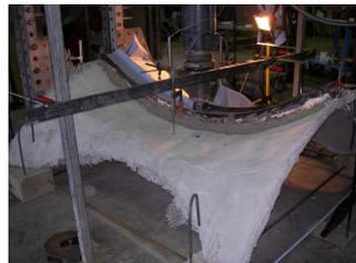
**Fig. 4** Test setup: line load on doubly curved shell
