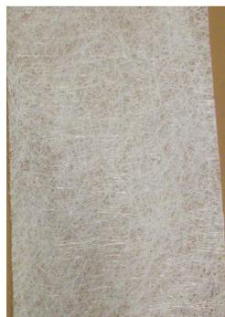
**Fig. 1b** Randomly oriented glass fibre textile
