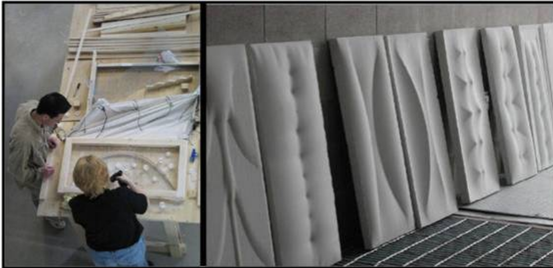
Fig. 1. Model formwork and completed plaster cast.
