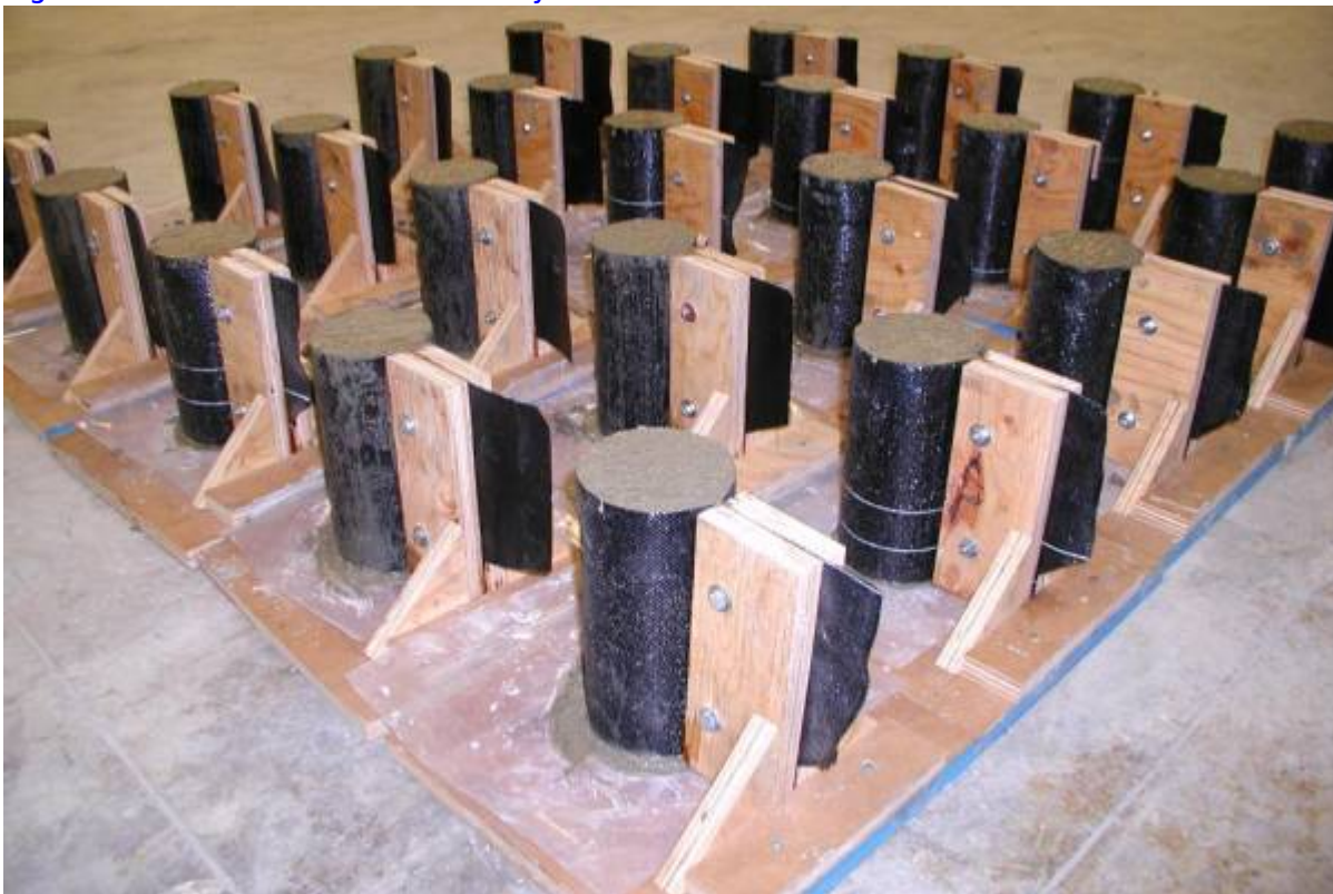
Figure 35: Fabric-formed cylinders after casting.
