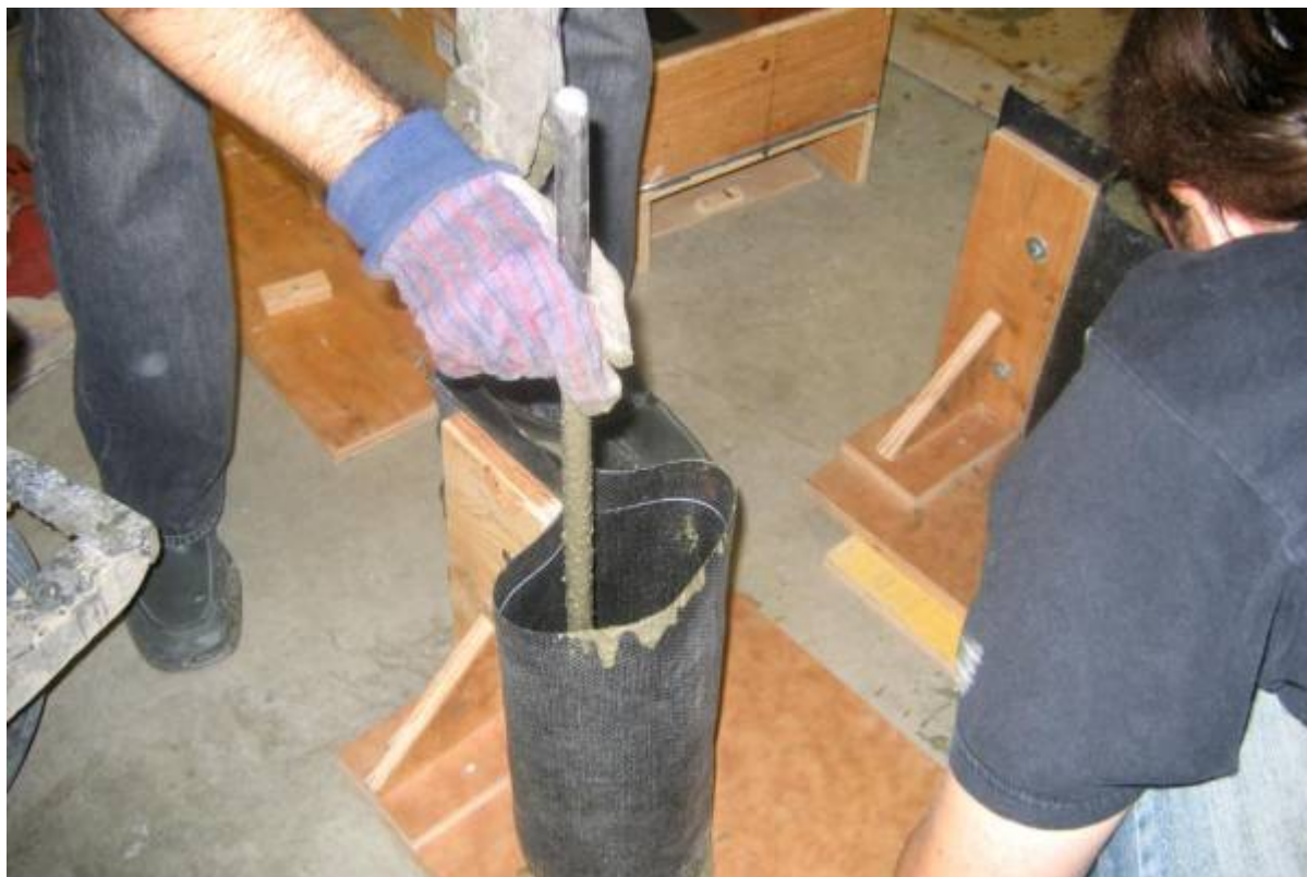
Figure 21: Compacting fresh concrete using the standard rod.
